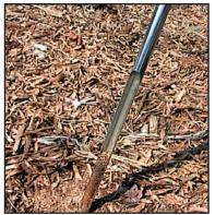
Figure 4. A small soil corer is ideal for quickly assessing soil moisture content.
